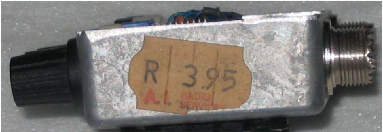
The and view show clearly how the components are above the level of the bottom of the box, filling the space of the raised lid. The switches have a total of less than 1/32" total clearance between the top and bottom of the case.
