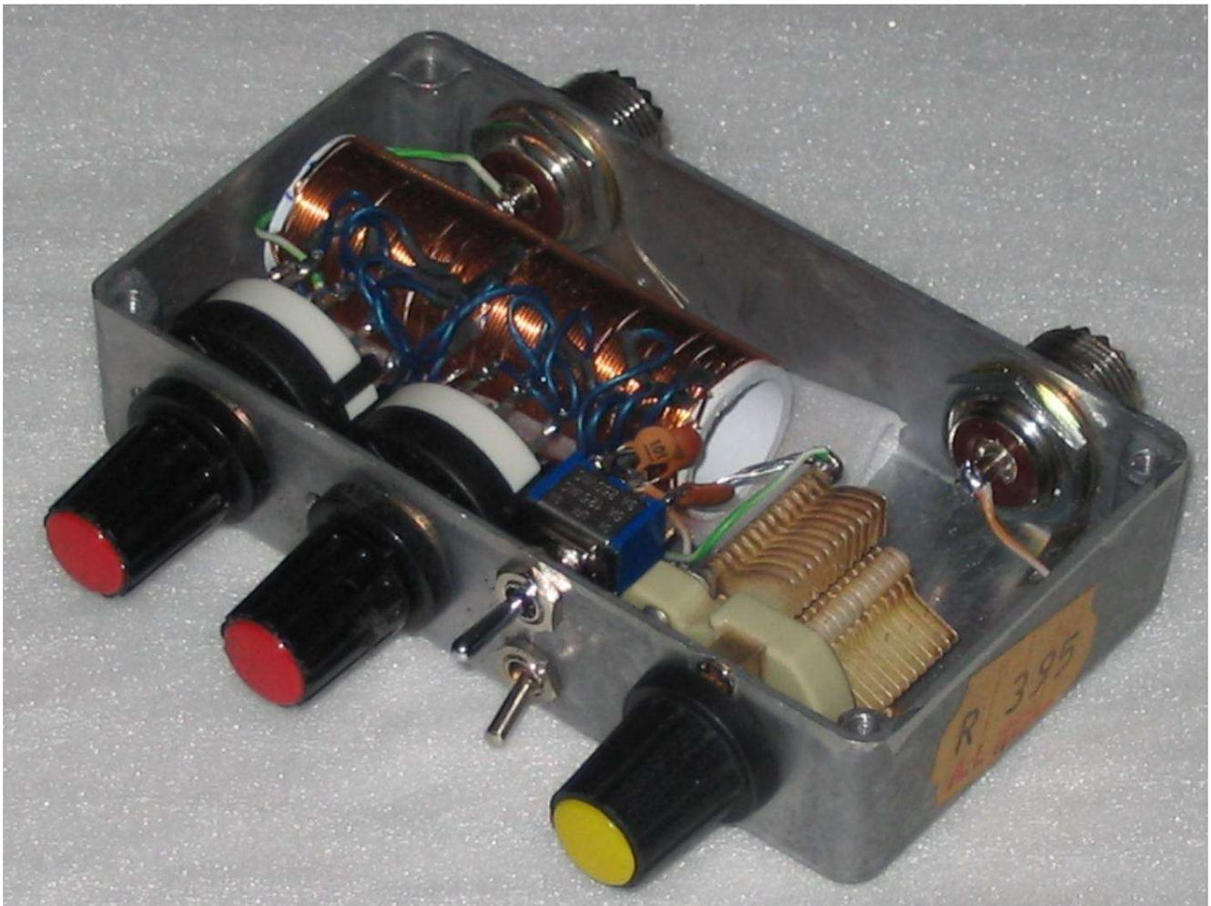
As you can see, the fit is fairly tight, in fact all the controls are touching each other, so there is no room for error when measuring before drilling.
