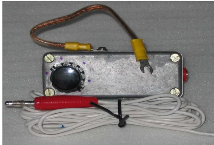
A counterpoise is most needed when running of internal batteries and using a “walkabout” antenna.
